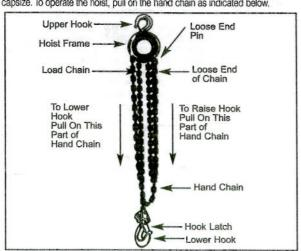
Operate the hoist with no load and then a light load of approximately 50 pounds (23 Kg.) times the number of load supporting chains to make sure it operates properly and the brake holds the load when the hand chain is released; then operate with a rated load as shown on the capacity plate.
